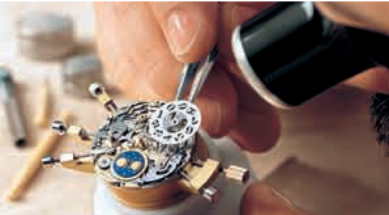
Traditional craft, innovative design: assembling an outsize date on a Langematik Perpetual watch
