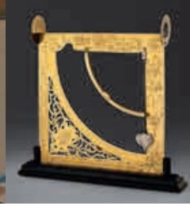
Mathematisch-Physikalischer Salon Research project "Shot at Noon – European Artillery Instruments c. 1500 to 1750": Gunner's quadrant (P. Puchner and C. Trechsler the Elder)
