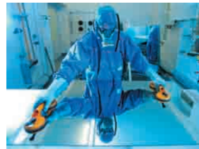
Mirror manufacturer Steffen Noack making historic mirrors using an amalgam of tin and mercury
