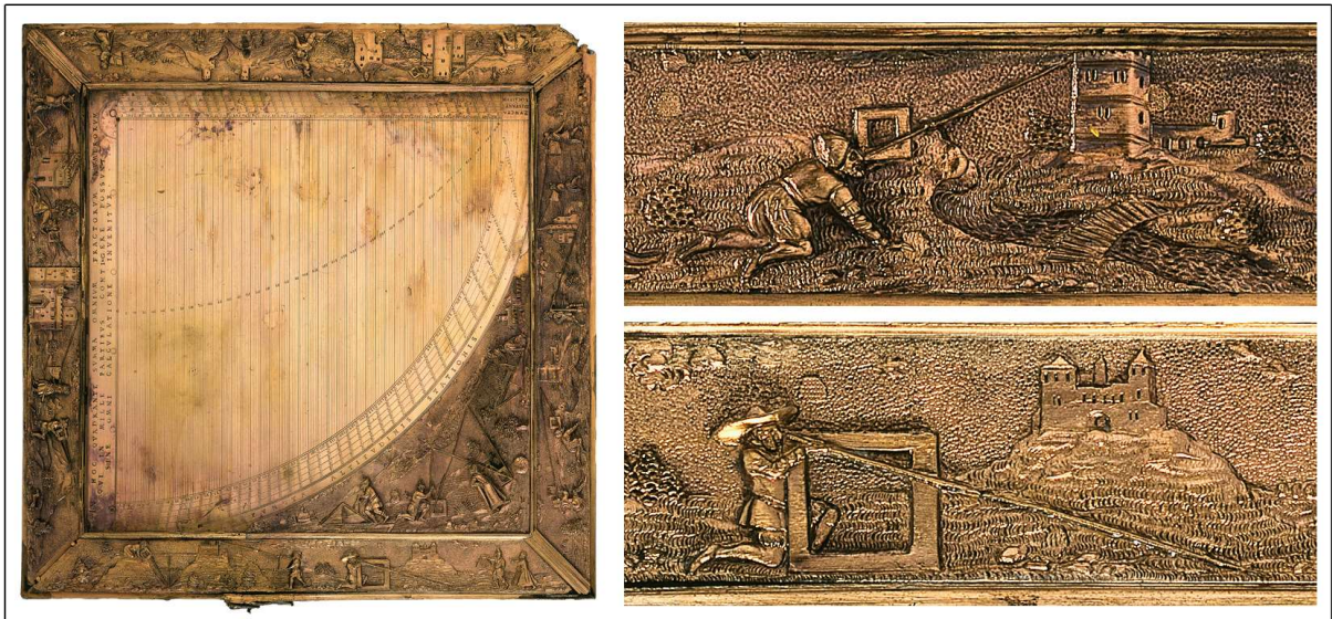
Links: Messquadrat (Quadratum Geometricum), Christoph Schissler, Augsburg, 1569, MPS Inv.-Nr. C I 1. Rechts: Details
